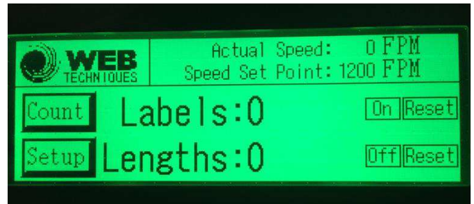
WT-30LCI Screen Demonstrating 1200 Feet Per Minute Speed Setpoint
