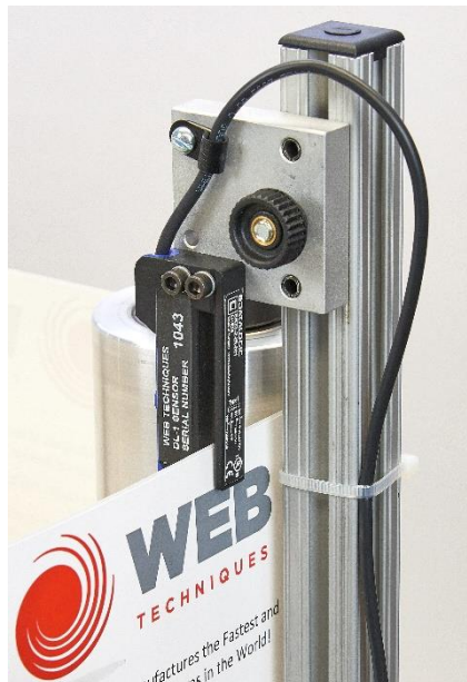
PC-30 Unit above, Photoelectric Sensor below
