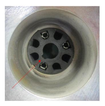
You do not need a tool to replace a strobe flash tube. You will want to use a shop towel and cover the tube, then wiggle it a bit while pulling it out. Use the same towel to cover the new bulb. You will want to line up the notch of the bulb with the socket, then push it into place. To remove and replace the cover you will only need a phillips screwdriver.
