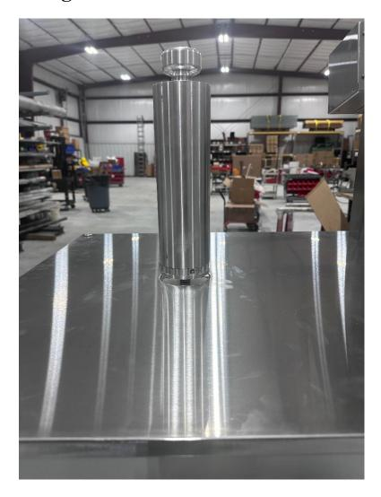
Note: Over time burrs can form on the drive shafts/coreholder shafts causing them to not sit flush with the top of the system. To remove any burrs from the drive shaft/coreholder shaft, follow the instructions below. If not removed this could cause the coreholder to get stuck in the system.
