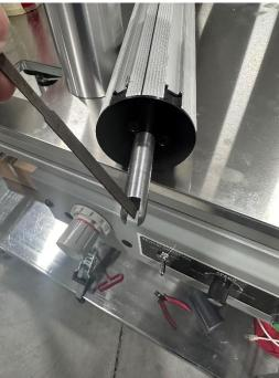
4) Place coreholder into system, if coreholder does not sit flush repeat the steps above.
